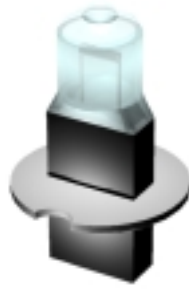
CAD Model of an automotive lightsource (type H3)
